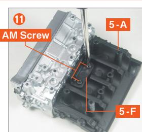
Hold **5-A** and **5-F** in place so they don't shift, align the screw holes, and secure them with two **AM screws**.
