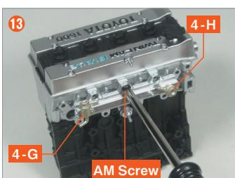
Secure the three screw holes of **4-F** with **AM screws**.
