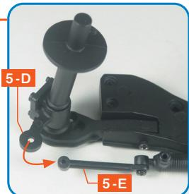
Align the screw holes of **5-E** and **4-B**, then secure them with an **AM screw**. Do not overtighten the **AM screw**.
