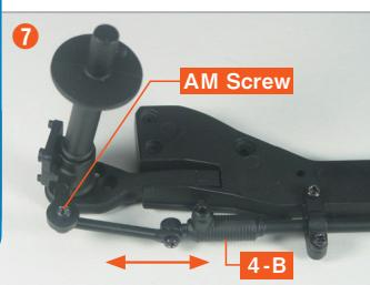
Fasten **5-E** from above with an **AM screw**. Be careful not to overtighten the **AM screw**, so that **4-B** can still move side to side.
