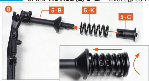
Pass the **Front Coil Spring 5-K** through the tip of **5-B** and insert the **Strut Upper Mount (L) 5-C**. While pressing **5-K**, guide the protrusion on **5-B** into the notch on **5-C**. When it meets resistance, slightly rotate **5-C** upward to secure it in place so it does not come off.
